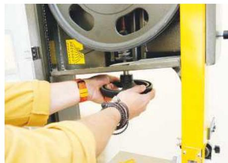
▲ The tensioning wheel is large and easy to operate
